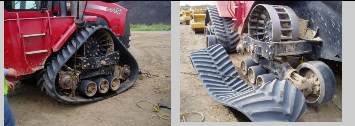
Using a boom truck to work track off the drive wheel and rear idler simultaneously
