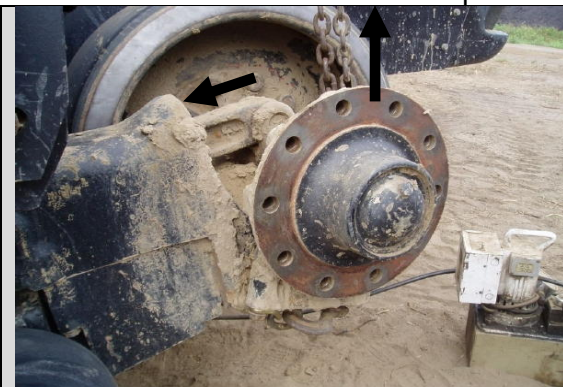
Chain attached to rear swing link bolt to force linkage inwards
