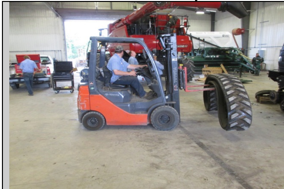
Using a forklift to safely move track to a suitable location
