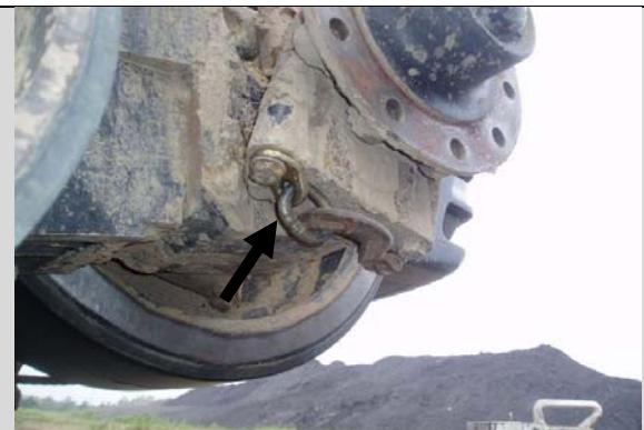
Gently pull up on the chain to cause cylinder to retract
