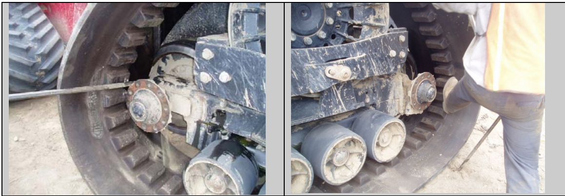
Track installation (Quadtrac shown above, however the same procedure applies to Rowtrac/T8 Smartrax)
