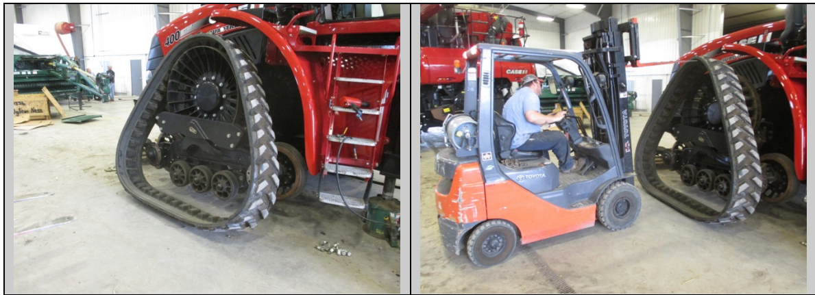
Using a forklift to lift track off the drive wheel
