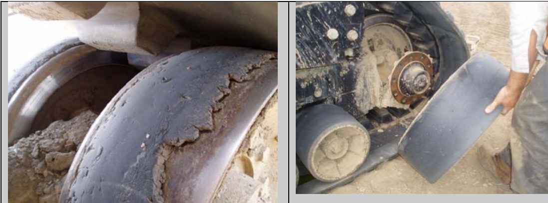
Idler Inspection (Quadtrac shown above, however the same procedure applies to Rowtrac/T8 Smarttrax)
