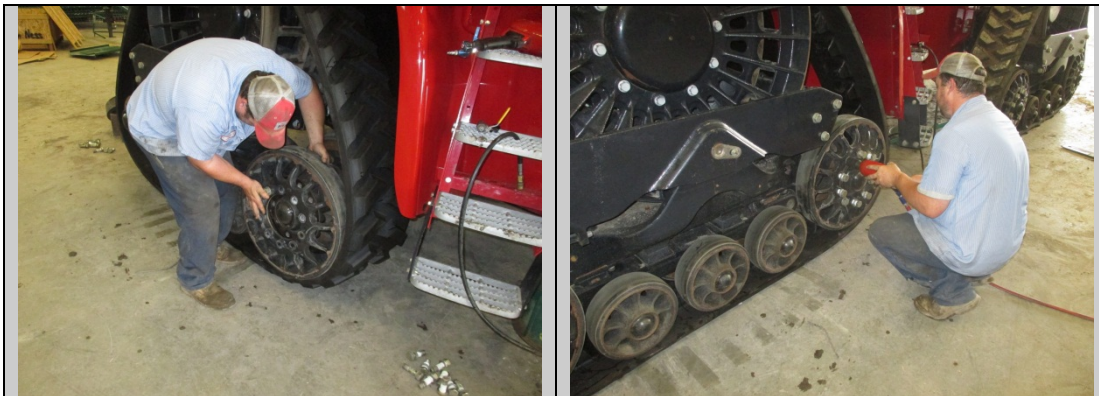
Idler Wheel installation
