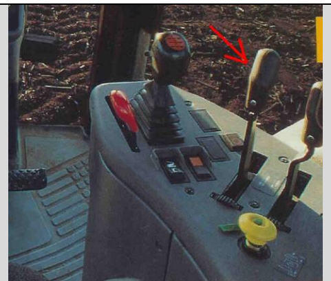
Caterpillar #1 Hydraulic Valve control
