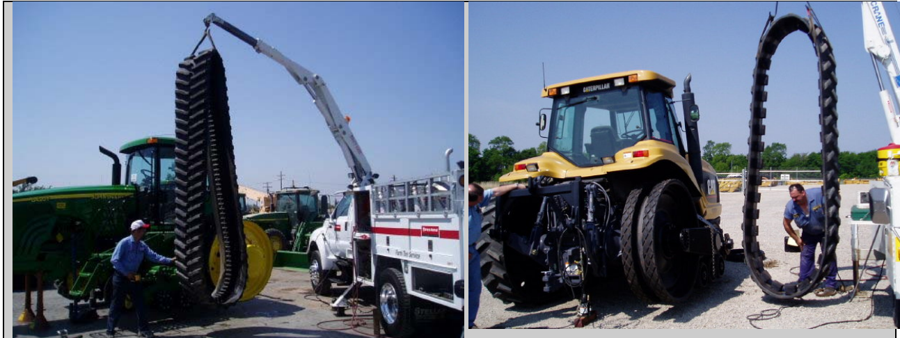
Using a boom truck to remove track (JD and Cat)
