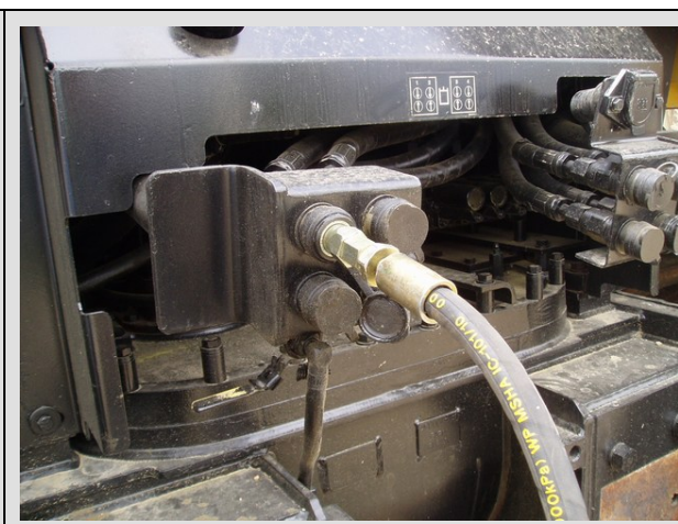
Opposite end connection to Implement Valve
