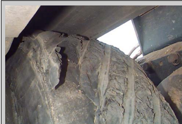
Drivewheel rubber damage – torn + chunking Wheel should be replaced
