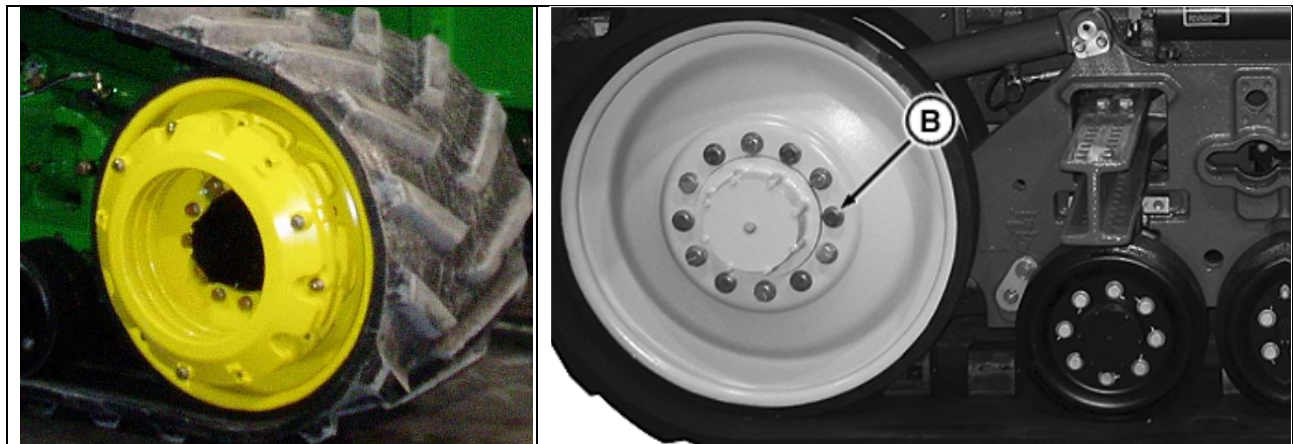
Remove Idler Weights on outboard side only Idler Cap Screws (B) Some bolts may also hold idler starter weight if equipped
