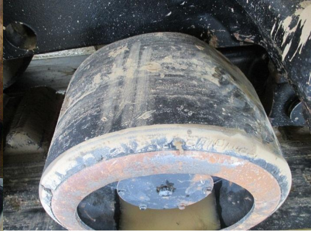
Midroller with flat spot. It should be replaced.
