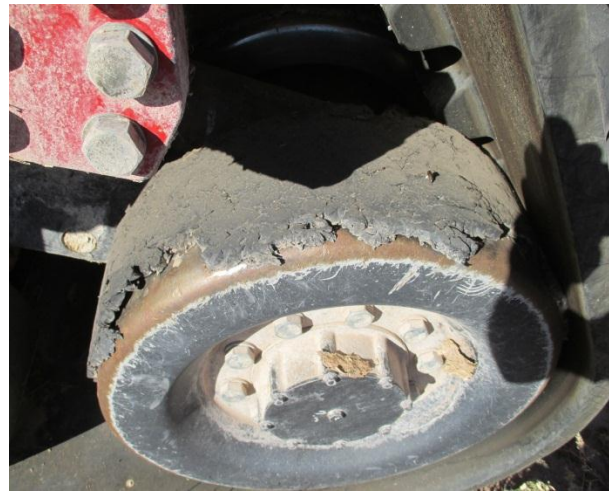
Idler with outside edge damage from rocks and debris.
