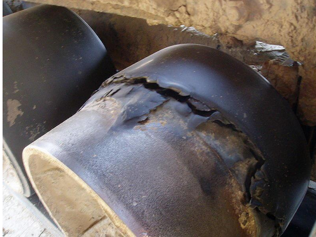
Midroller with more than 1/3 of polyurethane coating missing. It should be replaced
