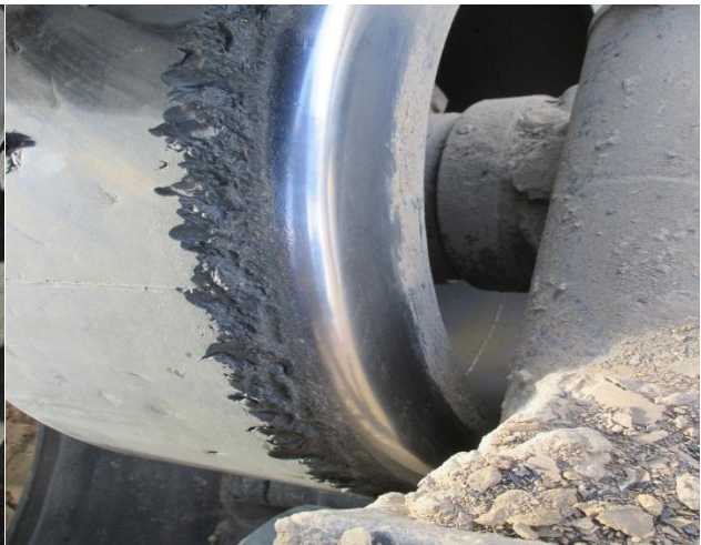
Idler with inside edge damage from misalignment and/or hard contact with drive lugs during turning
