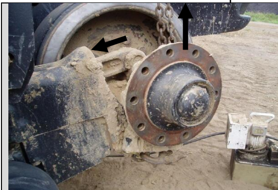
Chain attached to rear swing link bolt to force linkage inwards
