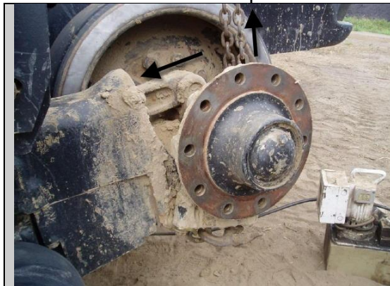
Pulling up on chain to retract tension cylinder to aid in track installation
