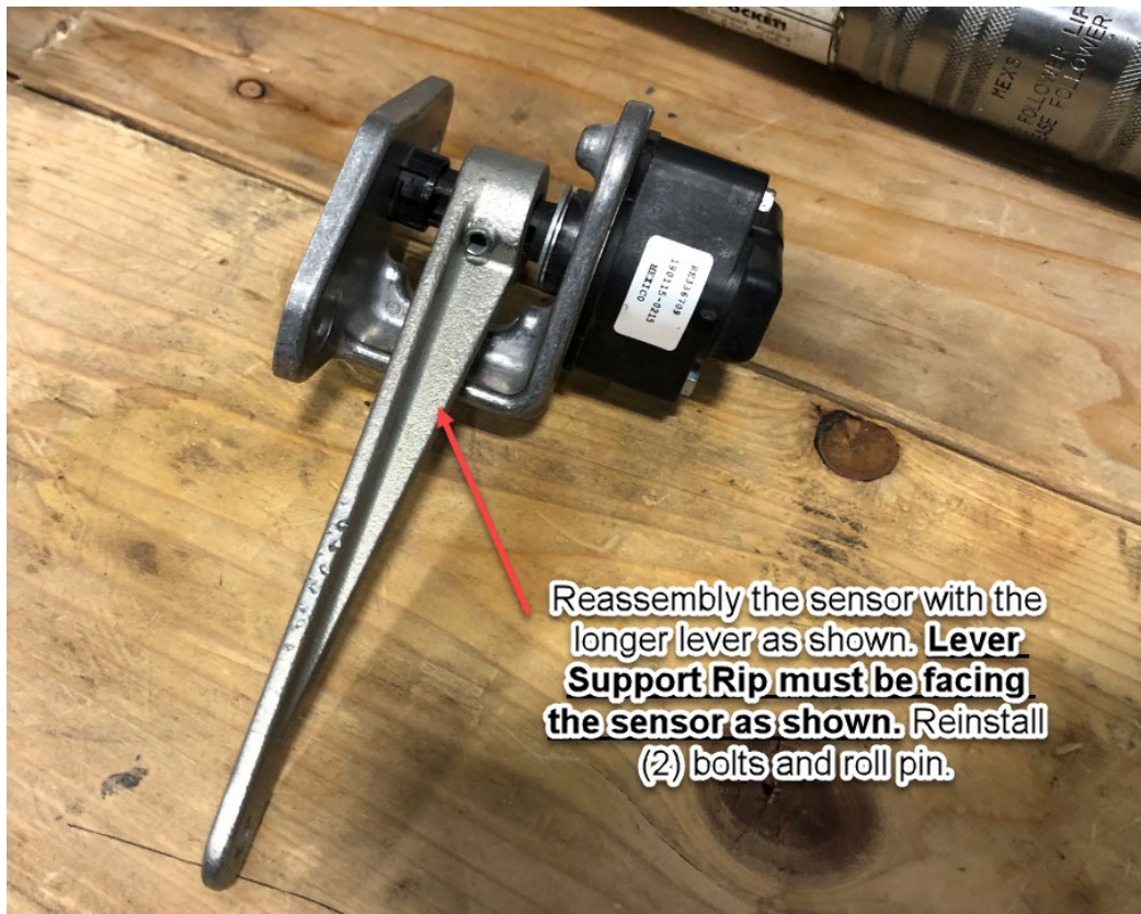
c.) Assembly of the revised sensor to the new mounting plate.
