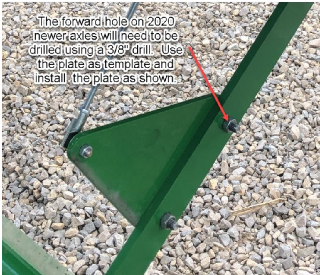
e.) Installed 2A-2629-100 kit on a 2018 or newer DB60-DB66 Planter
